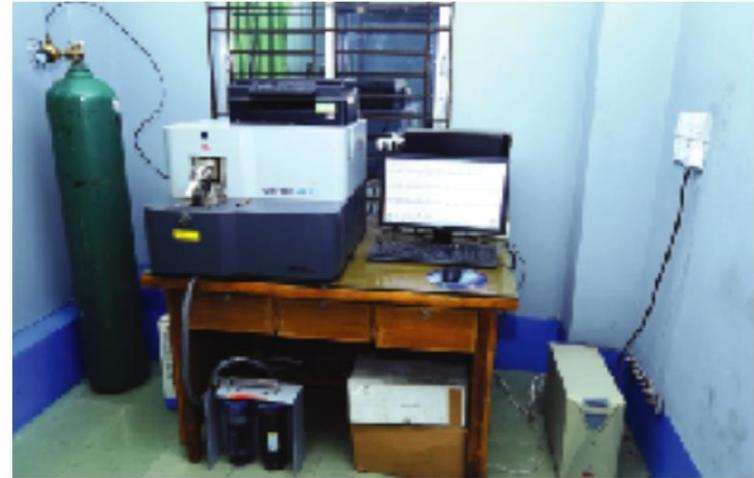
We have a sophisticated Chemical Lab to analyze the chemical composition of incoming raw materials (known as Billet) & the finished products. The main objective of the chemical analysis is to determine the existing percentage of Carbon (C), Silicon (Si), Manganese (Mn), Sulphur (S), Phosphorous (P) etc. in raw materials and in our finished products.
